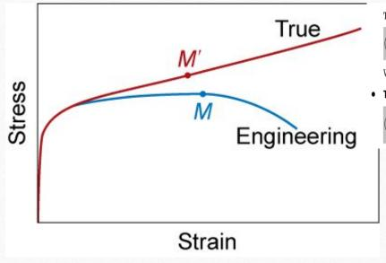
The true stress is defined as the ratio of the load to the cross section area at any instant.
