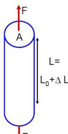
Load can be applied to the material by applying axial forces:
